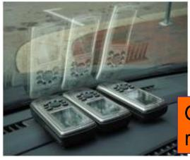
Portable Emissions Measurement System (PEMS) CO<sub>2</sub>, CO, HC, NO<sub>x</sub>
